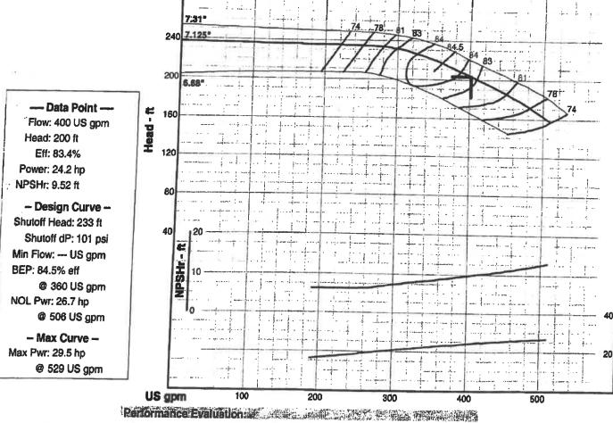
Flow Speed Head **Pump** Power **NPSHr** US gpm nom. %eff hp ft 480 1770 169 78 26.2 11.7 400 1770 200 83.4 24.2 9.52 320 1770 224 83.8 21.5 7.62 240 1770 231 76.5 18.2 6.06 160 1770
